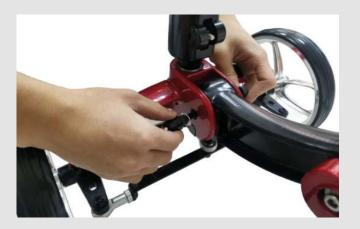
2. Adjusting handle bar (A) assembly – Attach the handle bars to the steering column. Ensure the brake line is not twisted around the bar. Place the handle bars at the desired height, making sure that the holes for inserting the locking knob (H) line up. Secure the handle bars with the locking knob (H). Twist the locking knob clockwise until fully tightened.
