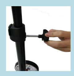
3. Insert the knee pad post into the receiver at the top of the knee walker frame. Lock the pad in place by inserting the locking knob (J) into the desired adjustable height hole making sure that the holes for inserting the locking knob line up. Twist the knob clockwise until it is fully tightened. Then insert the pin (F) and lock.
