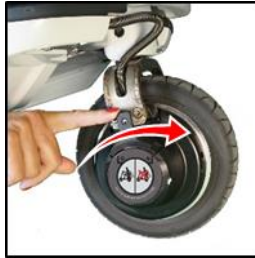
Figure 51 Releasing the freewheel
