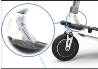
Figure 22 Steering Rod angle adjustment screws
