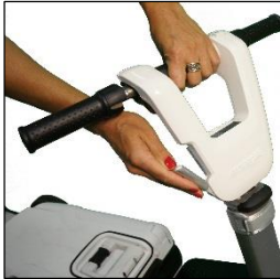
Figure 19 Driving Console tilt lever
