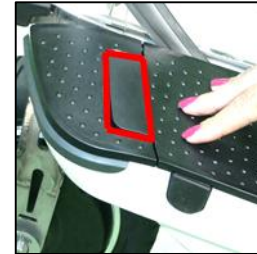
Figure 56 - battery release button
