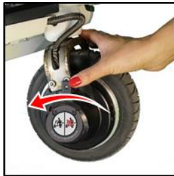
Figure 52 Securing the freewheel
