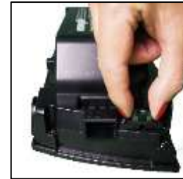
Figure 65 Replacing a blown fuse
